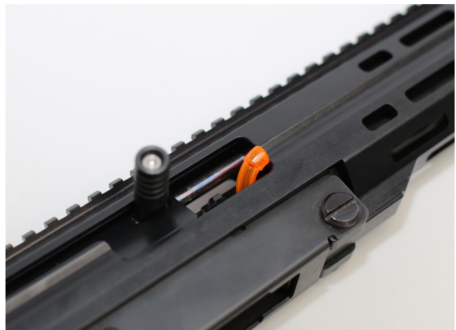
Use a chamber flag to prevent the bolt from closing completely
