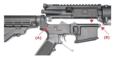
2. Unlock Safety Bail on Upper Receiver and Slide Retaining Block Forward.
