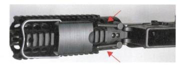
6. Slide Retaining Block Down and Lock Safety Bail Into Place.
