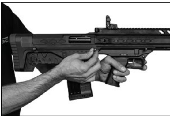
4) Pull the Upper Receiver Pivot Pins and handguard pivot pin to take out
