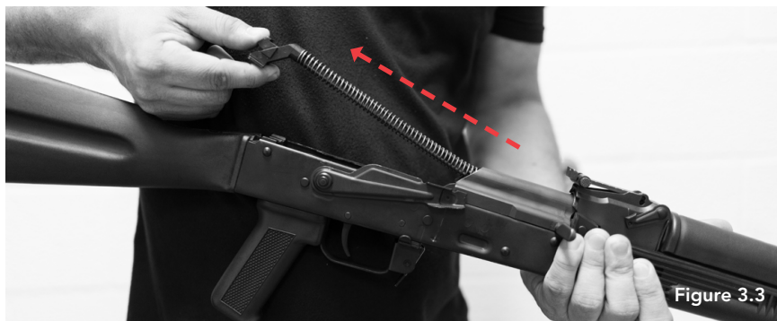
Figure 3.3 — Detaching The Recoil Spring Guide Assembly
