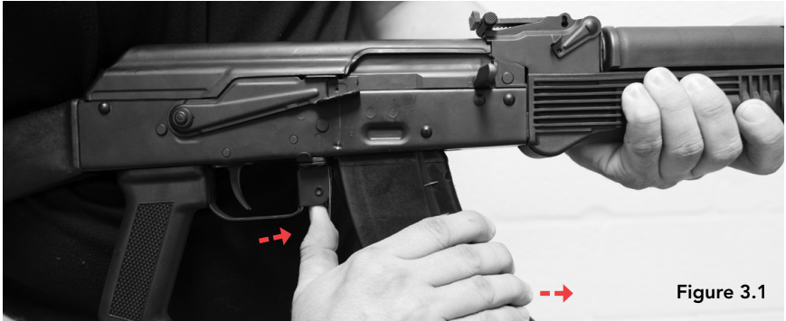
Figure 3.1 — Detaching The Magazine
