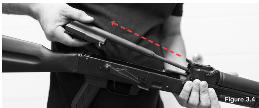
Figure 3.4 — Detaching The Bolt Carrier And The Bolt
