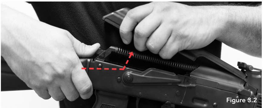
Figure 3.2 — Detaching The Receiver Cover
