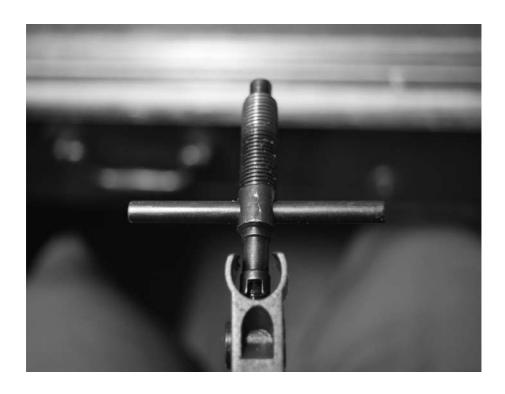
Use the Sight Adjustment Tool to adjust the elevation as seen in this picture.
