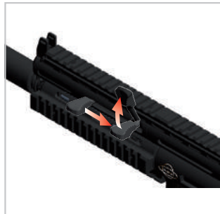
2. Pull the cocking lever back until it stops and hold it in this position
