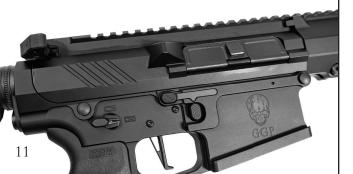
2.) Press magazine release button and pull the magazine down to remove it from the rifle.
