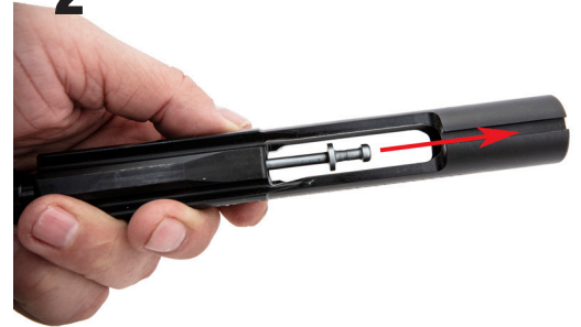
2. Remove the Firing Pin.
