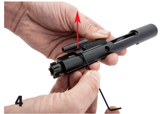
4. Inspect the Cam Pin for wear.
