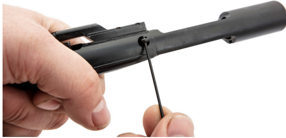
1. Remove the Firing Pin Retainer.
