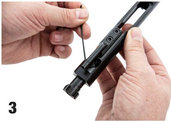
1. Remove the Firing Pin Retainer.
