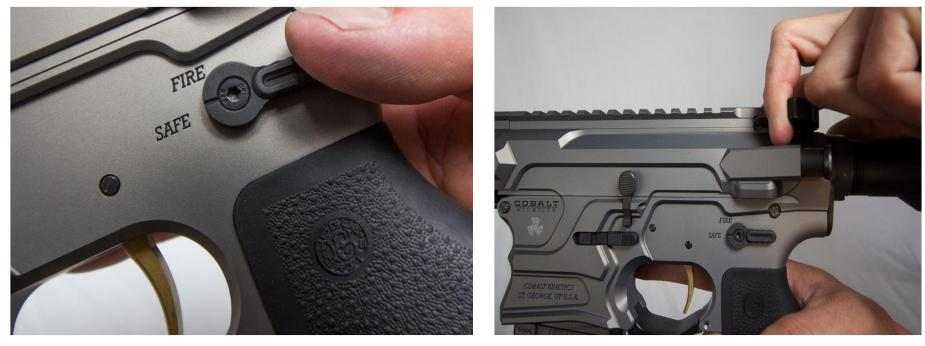
WITH THE MUZZLE POINTED DOWN RANGE AND THE WEAPON SHOULDERED, ALIGN THE SIGHTS WITH YOUR TARGET OF CHOICE. ROTATE THE SELECTOR LEVER TO THE "FIRE" POSITION AND PLACE FINGER ON TRIGGER. WHEN THE SIGHTS ARE PROPERLY ALIGNED ON TARGET, LIGHTLY PRESS THE TRIGGER AND FIRE THE WEAPON.
