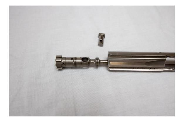
PRESS IN THE REAR OF THE EXTRACTOR AND USE A SMALL PUNCH TO PUSH OUT THE EXTRACTOR PIN. LIFT THE EXTRACTOR FROM THE SLOT ON THE BOLT. BE AWARE THERE IS A SMALL SPRING AND INSERT PRESSED INTO THE UNDERSIDE OF THE EXTRACTOR. CARE SHOULD BE TAKEN TO NOT LOSE THIS COMPONENT.
