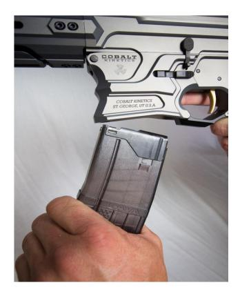
WITH THE SELECTOR IN THE "SAFE" POSITION, PULL THE CHARGING HANDLE FULLY TO THE REAR AND RELEASE, ALLOWING THE BOLT CARRIER ASSEMBLY TO TRAVEL FORWARD UNDER POWER OF THE BUFFER SPRING. THIS ACTION WILL STRIP A LIVE ROUND OF AMMUNITION FROM THE MAGAZINE AND PLACE IT IN THE CHAMBER OF THE RIFLE. YOUR WEAPON IS NOW LOADED AND READY TO FIRE.
