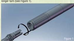
To remove the silencer from the flash hider, simply reverse the above procedure.
