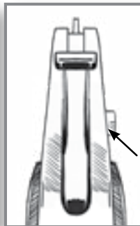
Safety in “ON FIRE” Position
