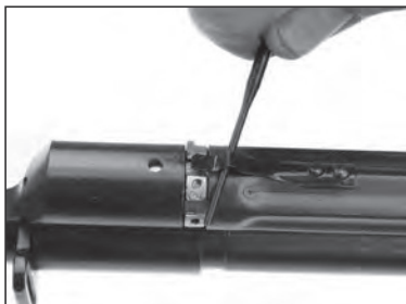
Fig. 6 - Lifting the spring securing pin
