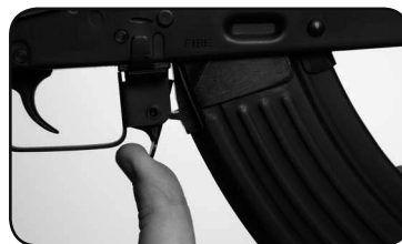
Picture #6 RELEASE MAGAZINE by pressing the magazine release lever forward
