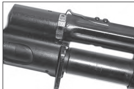
Fig. 7 - Regulator in position 2 - normal conditions
