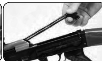
Picture #13 Remove the recoil spring
