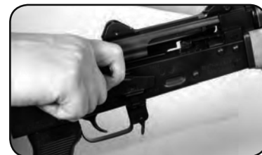
Picture #7 Pull Bolt charging handle all the way back to expose the chamber
