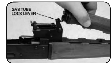
Picture #16 Remove gas tube (upper hand guard assembly)
