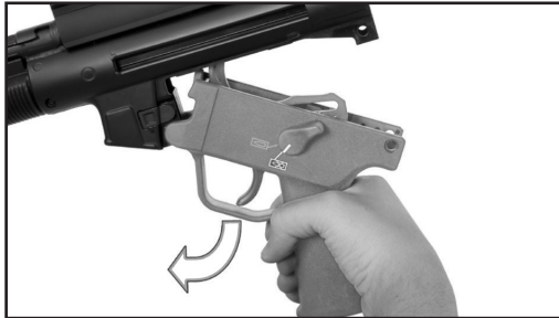
Fig. 36 – Remove pistol grip
