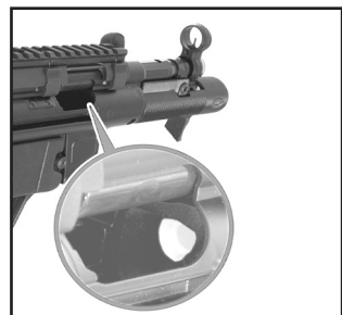
Fig. 22 – Check the chamber
