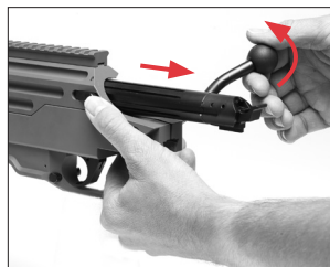
Rotate the bolt handle up and pull it to the rear.
