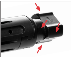
Lightly lubricate the bolt's three locking lugs and the rear locking surface.
