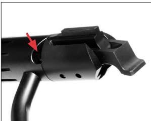
Lightly lubricate the bolt cocking surface.
