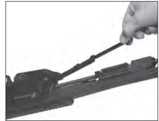
Pull the action bars forward and out of the receiver.
