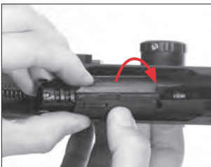
Carefully rotate the bolt out of the receiver.
