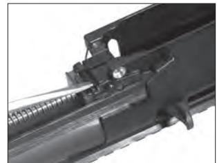
Release the bolt lock spring.
