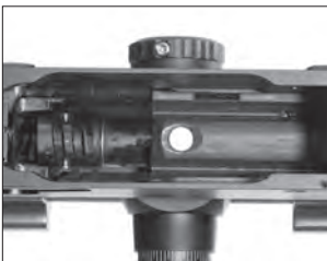
The bolt shown correctly positioned.
