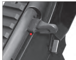
Verify the bolt is fully forward.
