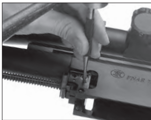
Tap out the pin from the left to the right side.
