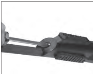
Carefully remove the forearm attachment nut with a screwdriver.
