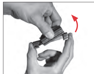
Compress the springs and separate the inertia block.
