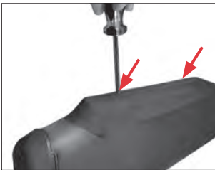
Carefully remove the two screws that attach the comb to the buttstock.
