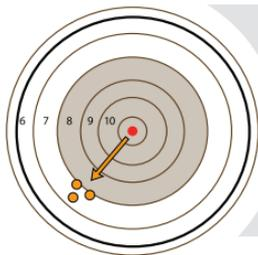
To place the center of the reticle (red) on the point of impact (orange), turn the elevation turret counter-clockwise to raise the point of impact. Then, turn the windage turret counter-clockwise to move the point to impact to the left.
