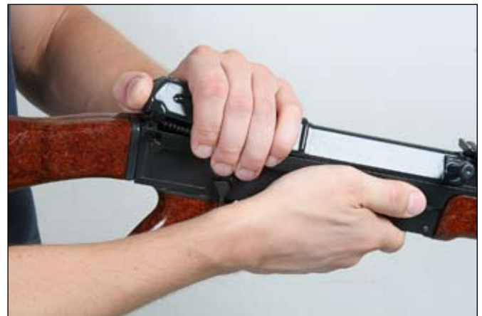
Fig. 29 Removing the return mechanism
