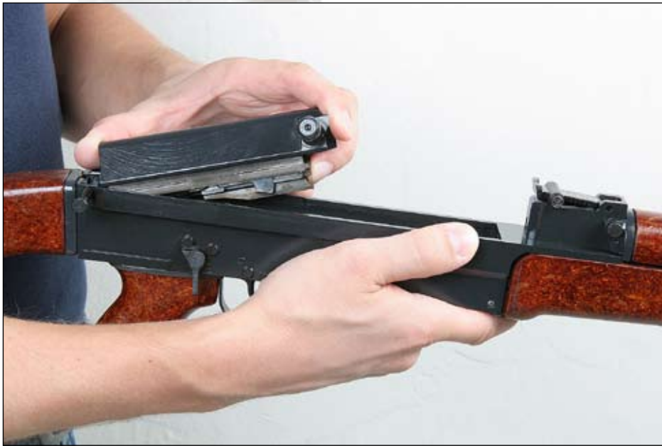
Fig. 30 Taking out the bolt
