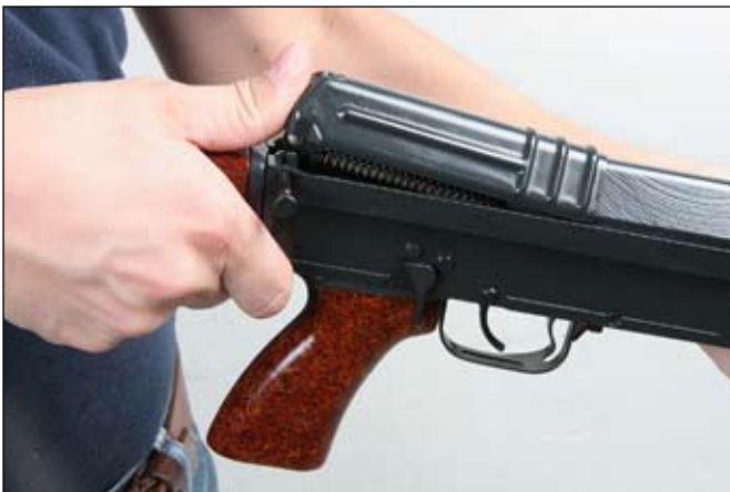
Fig. 28 Removing the return mechanism
