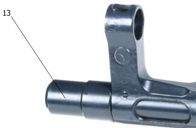
Fig 5. Barrel extension /side view/ 13 - barrel extension
