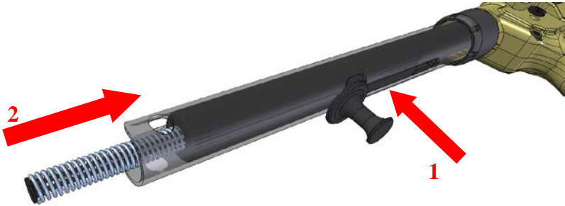
Figure E-2: Bolt Assembly in Receiver with Recoil Spring
