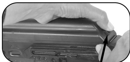
Spring loaded release button.
