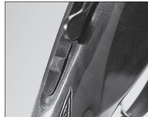
The thumb "safety" shown in the forward "off safe" position.
