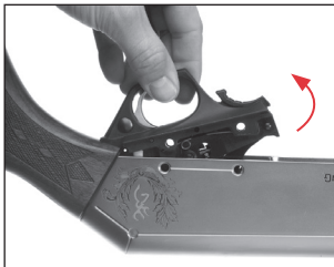
Lift the trigger group from the receiver.
