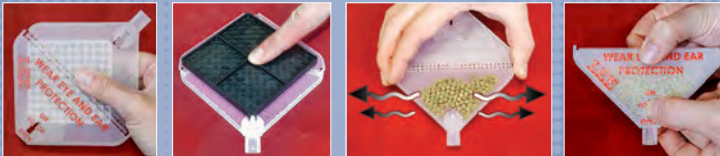
Unfold tray and place on top of box of 100 primers. Flip tray over to deposit the primers. Shake tray to upright all the primers. Fold and close cover. Slide the flow control to LOCK.
