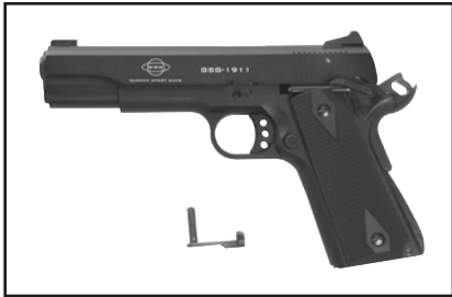
Fig. 1: Slide stop removed
