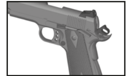
Fig. 1: Grip safety is cocked
