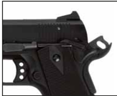
Fig. 2: safety is deactivated, Pistol is cocked and ready for firing
