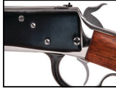
Hammer on the half-cocked position
