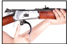
Swinging the Finger-Lever
