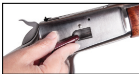
Gun being loaded through the loading port
