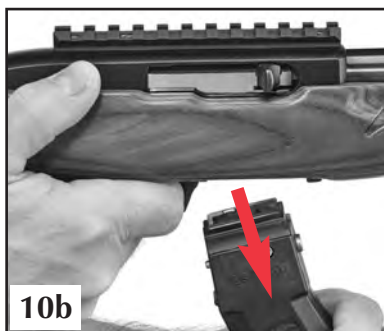
Figure 10. The safety should be “on” when the magazine is being removed or inserted. Move the magazine release forward (Figure 10a) and draw the magazine out by grasping it between your thumb and forefinger and draw it out of the firearm (Figure 10b).
