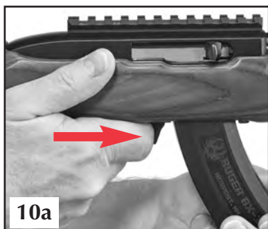
Figure 10. The safety should be “on” when the magazine is being removed or inserted. Move the magazine release forward (Figure 10a) and draw the magazine out by grasping it between your thumb and forefinger and draw it out of the firearm (Figure 10b).
