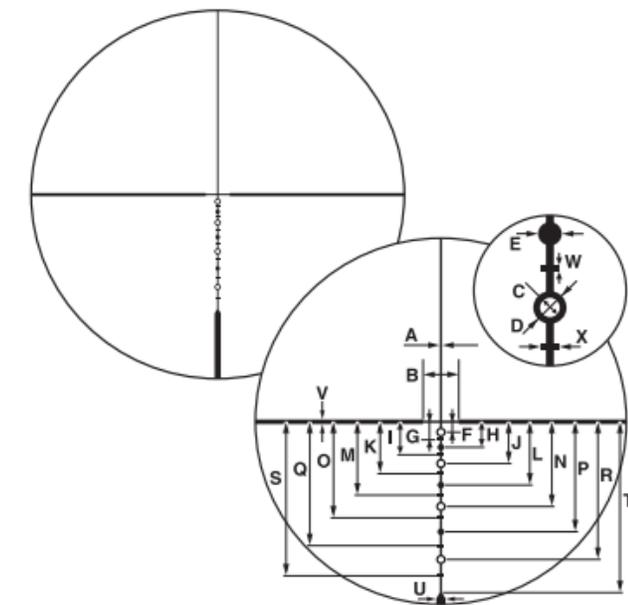
Letters A to X in the diagram above refer to the reticle subtensions of units A to X shown on the table to the right.
