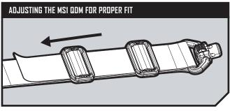
Adjust the length of the sling such that the Slider remains accessible by your non-firing hand both when tight (slung) and loose (rifle in use). After you have determined the proper length for your MS1 QDM Sling, run the tail end back through both of the Fit Buckles provided. Double back any excess material and trim only if necessary.
