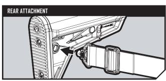
Grip both QDM Actuation Surfaces with finger/thumb and push Rear QDM into Stock QD Socket. Use socket on side facing away from user.
