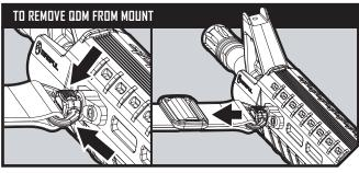
Grip both actuation surfaces with finger/thumb and pull from socket.
