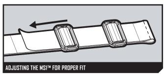
Adjust the length of the sling such that the Slider remains accessible by your non-firing hand both when tight (slung) and loose (rifle in use.) After you have determined the proper length for your  $MS1\ Sling$ , run the tail end back through both of the  $Fit\ Buckles$  provided. Double back any excess material and trim only if necessary.
