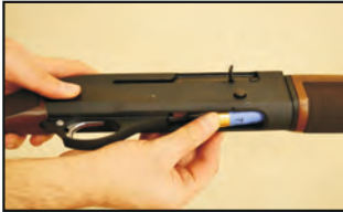
2- The bolt will return to the closed position.
