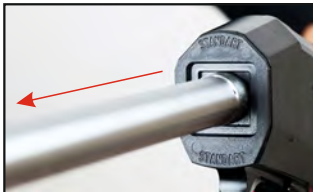
5. Remove the "STANDART" marked shim from the action tube. (Your shotgun comes with "STANDART" shim that gives a no cast stock.)
