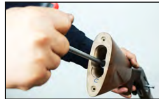
12. Screw the stock using a socket wrench.
