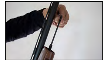
2. First remove the magazine cap. Cup upward and remove the plug. Re-install the magazine cap.
