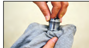
8- Clean the inside and the outside of the piston using the same method.
