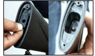
9. Insert the cast plate (L) into the stock while the letter "L" is visible. (Your shotgun comes with "R" visible cast plate that gives no cast stock when used with "STANDART" drop shim.)
