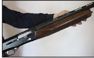
10. Tighten the magazine cap in front of the forearm by turning it clockwise.
