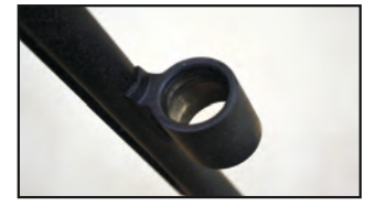
5- O-ring is located inside the barrel ring so it's not visible on magazine tube.
