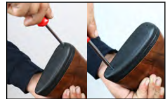
13. Screw the butt pad screws by using a phillips screwdriver.
