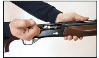
2. Pull the bolt handle to the rear to eject the round from the chamber.
