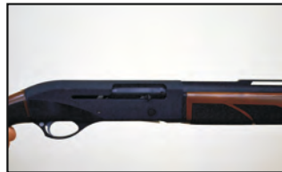
2- The bolt will return to the closed position.
