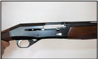
4. The bolt must be allowed to close forcefully to fully chamber the round. One cartridge from the magazine is now chambered. You can now place another cartridge into the magazine to replace the chambered round.
