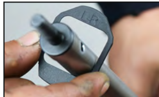
6. Place the cast shim to the back of the receiver while the marking "L-R" is visible.
