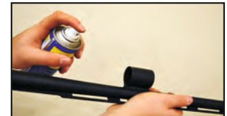
9- Clean the gas ports on the inside of the barrel lug. Clean inside of the barrel lug.
