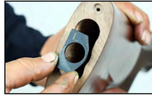
9. Insert the cast plate (L) into the stock while the letter "L" is visible. (Your shotgun comes with "R" visible cast plate that gives no cast stock when used with "STANDART" drop shim.)
