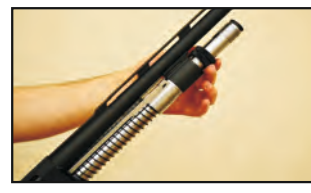
3- (CZ 712 G2 &amp; CZ 720 G2 Models Only) Unscrew the supporter nut off the front of the magazine tube.
