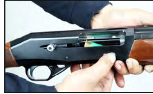
3. Push the bolt release button and engage the safety.
