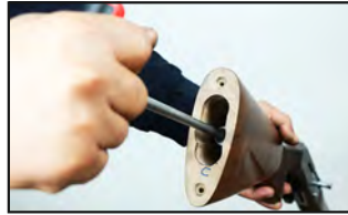
2. Unscrew the stock bolt using a socket wrench.
