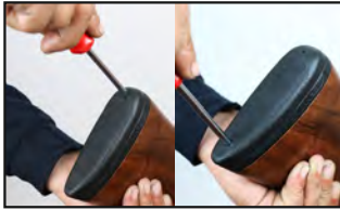
1. Unscrew the butt pad screws by using a phillips screwdriver and take the butt pad out.
