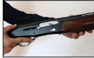
1. After filling the magazine push the cartridge drop lever to allow the cartridge to drop on the carrier.
