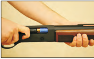
1- Pull the bolt handle to the rear to eject the round from the chamber
