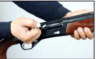
1. Pull the bolt handle rearward until the bolt locks open.
