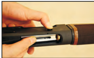
3- Hold the carrier down and depress the feed latch. 4- A cartridge will drop down to your finger on the carrier. Take out the cartridge. Repeat this operation until the magazine is empty. Depress the cartridge drop lever at the back of the carrier and pull the bolt handle rearward until the bolt locks open, demonstrating that the gun is completely unloaded.
