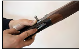
3. Push the carrier and depress on the back of the bolt release button. Cartridges will drop down to your finger on the carrier. Take out the cartridge. Repeat this operation until the magazine is empty. Depress the cartridge drop lever at the back of the carrier and pull the bolt handle rearward until the bolt locks open, demonstrating that the gun is completely unloaded.
