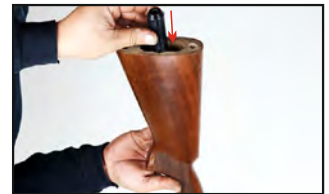
11. Put the stock supporter tube into the stock.
