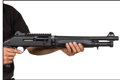
2) Slide The fore-end off the magazine tube
