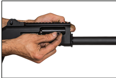
3) Move back the mechanism and ensure that cocking lever comes to the middle of the mechanism bearing; then, pull out and remove the cocking lever. During this operation, hold the cocking-bar so that the spring doesn't push it forward
