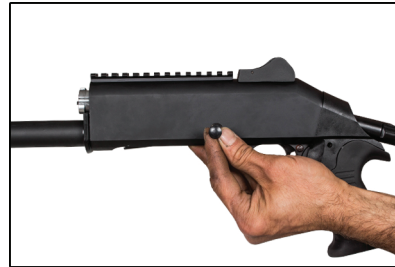
4) Take out the trigger group anchor pin.
