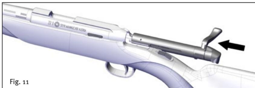
3. Hold the bolt by the bolt handle and insert it into the housing (Fig. 11).
