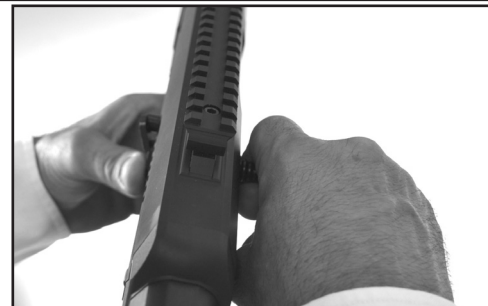
Fig. 18-2 Pull charge handle and push bottom of bolt hold open lever.
