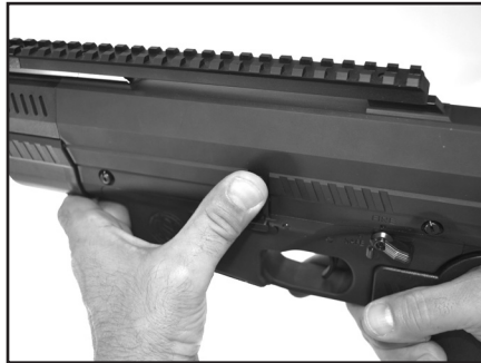
Fig. 18-4 Closing bolt by pressing top tab of bolt hold open lever
