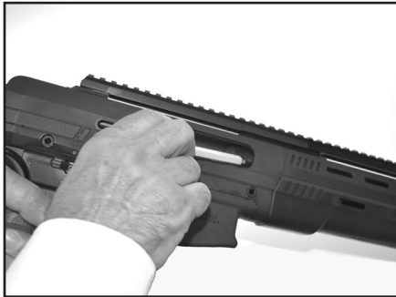
Fig. 18-3 Visually and physically inspect that chamber is empty.
