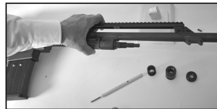
Fig. 18-10 Spring loaded nut and LH thread lock nut removed
