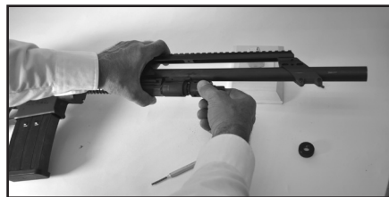
Fig. 18-9 Remove spring nut & O-ring sleeve
