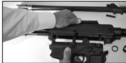
Fig. 18-16 Pull lower receiver down
