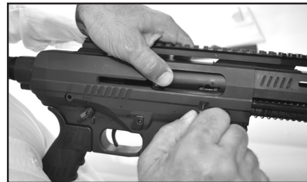
Fig. 18-13 Remove charging handle
