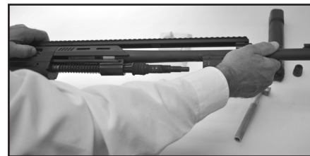
Fig. 18-11 Move bolt back and remove barrel
