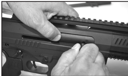
Fig. 18-12 Align handle with arch in slot
