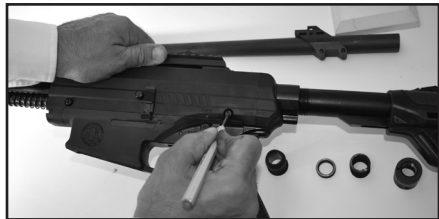
Fig. 18-14 Push rear detent pin toward flanged end
