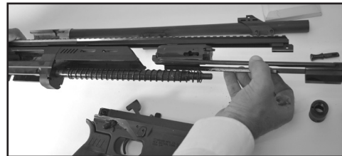
Fig. 18-17 Bolt, carrier and recoil spring can be removed
