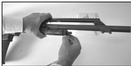
Fig. 18-8 Remove LH thread lock nut
