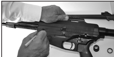
Fig. 18-15 Push front detent pin toward flanged end
