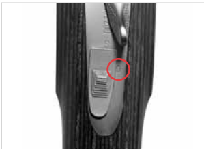
The "safety"/selector in the over barrel first position.
