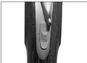
The “safety”/selector in the off safe position. The “S” is not visible.
