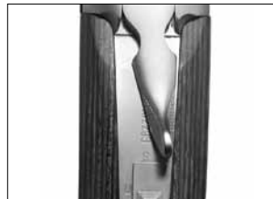
When closed, the top lever may still be slightly to the right of center. This is normal.
