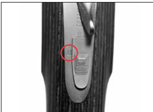
The "safety"/selector in the under barrel first position.
