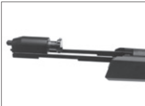
Position the bolt assembly on the slide arms.
