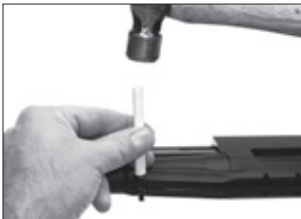
Carefully tap the rear sight base in the dovetail to adjust for windage.
