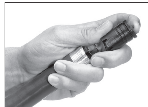
Carefully remove the magazine spring retainer.
