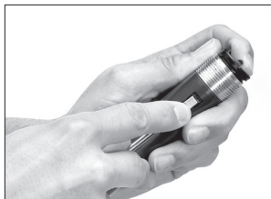
Depress the magazine spring retainer tab.
