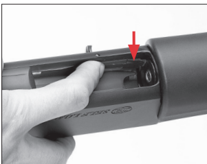
Press in on the shell stop to unload shells from the magazine.
