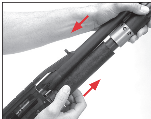
When installing the barrel and gas piston, you may need to lift the piston sleeve slightly.
