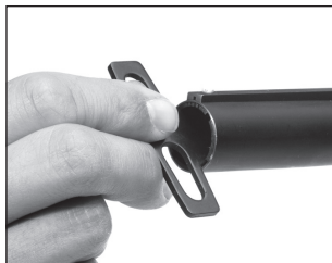
Use the choke tube wrench to change choke tubes.
