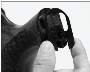
Install the selected shim onto the buttstock.
