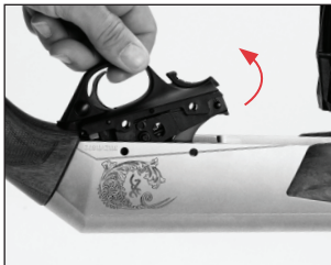
Lift the trigger group from the receiver.
