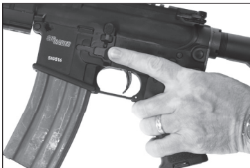
MAG CATCH BEING DEPRESSED LEFT AND RIGHT SIDE
