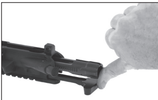
REINSTALLATION OF THE BOLT CARRIER ASSEMBLY TO UPPER RECEIVER
