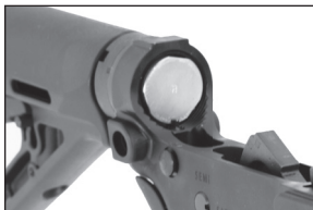
BUFFER HELD INTO RECEIVER EXTENSION
