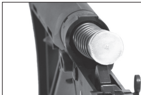
ACTION SPRING AND BUFFER STARTED INTO RECEIVER EXTENSION
