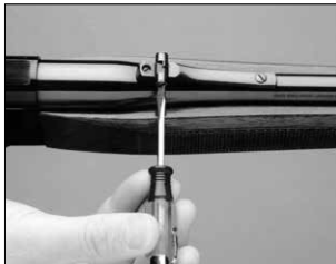
Rear sight horizontal adjustment.
