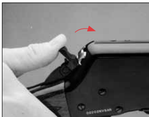
The folding hammer rotates forward for additional safety.
