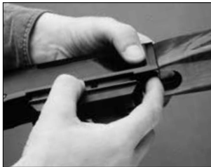
Press down on the magazine release.
