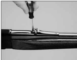
Rear sight elevation adjustment.
