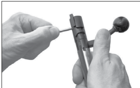
Figure 3, Cocking the bolt
