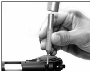
Gently tap the rear sight to adjust windage.
