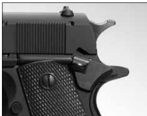
The hammer in the dropped position.
