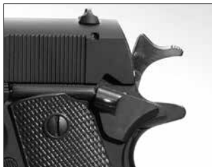
The hammer in the half-cock position.
