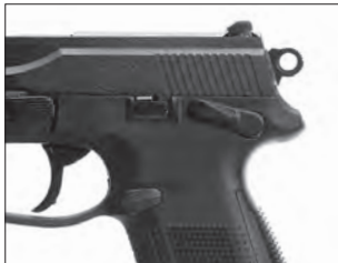
Hammer decocked for double-action firing
