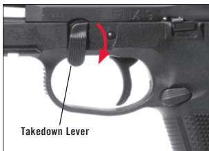
Rotate the takedown lever downward.
