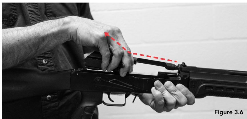
Figure 3.6 — Detaching The Bolt Carrier And The Bolt
