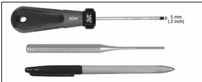
Figure 39 – Screw driver, punch and pen body (the point of a pen body can be used as an alternative to a metallic punch)
