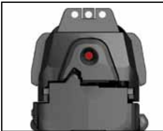
Figure 11 – Firing pin cocked
