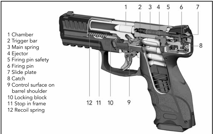
Figure 3 – VP Series Cutaway View
