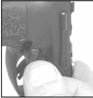
Figure 45 – Turning the pistol so it is facing down may make the installation of the push button easier
