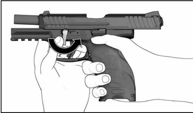
Figure 28 – Pivot the disassembly lever counter clockwise
