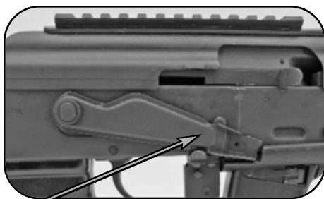
Safety lever in lower or “FIRE” position. Pulling the trigger when the safety lever is in the lower position will result in the pistol firing if there is a round in the chamber! Exercise extreme caution when handling pistol in this condition.
