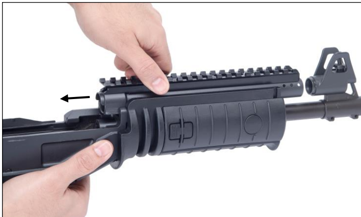
Figure 4-5: Gas Cylinder Disassembly
