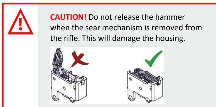
Figure - TAVOR® 7 Sear Mechanism Removal
