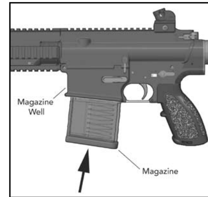
Fig. 30 – Inserting Magazine into the Rifle
