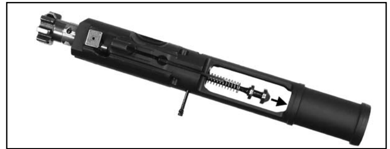
Fig. 40 – Removing the Firing Pin and Firing Pin Spring from the Bolt Assembly
