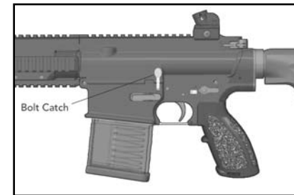
Fig. 31 – Depressing Bolt Catch to Chamber a Cartridge
