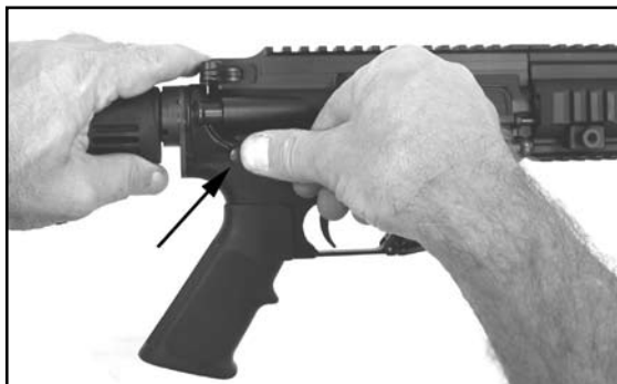
Fig. 99 – Completing the installation of the MR556A1 Upper Receiver on the Lower Receiver
