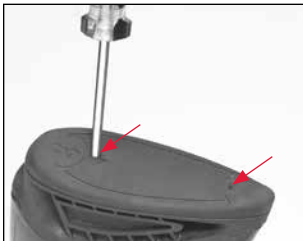
Locate the two entry holes in the recoil pad.
