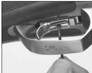
Remove the trigger retaining screw.
